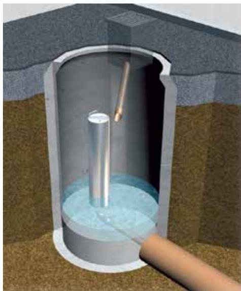
*Schematic of a HydroFlush siphonic chamber (courtesy Hydrok UK)*
