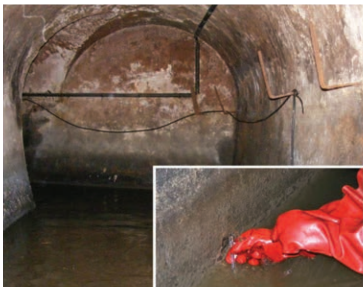
Sampling biofilm from a sewer wall in Nantes, France. Courtesy of Catherine Biggs.
